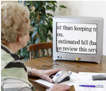
Figure 7a: The MonoMouse™ fits comfortably into the patient's hand and the simple one-touch blue button is highly visible. The slightly larger than average size of the MonoMouse is easier to use than a standard-sized optical mouse, which makes it attractive to those who find handling an issue.
