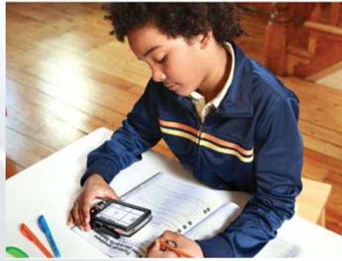
Figure 5c: (left) Bierley's Explora Plus™ is a portable electronic magnifier measuring 77 x 85 x 25mm and weighing 108g. Magnification is provided up to 9x and there are options such as image freeze, and contrast reversal
