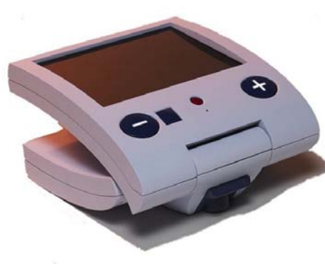
Figure 5a (above): FarView by Optelec: Distance and Near viewing Options. Up to 24x magnification with up to 4 hours continuous use from fully rechargeable battery
