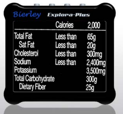
Figure 5c: (left) Bierley's Explora Plus™ is a portable electronic magnifier measuring 77 x 85 x 25mm and weighing 108g. Magnification is provided up to 9x and there are options such as image freeze, and contrast reversal
