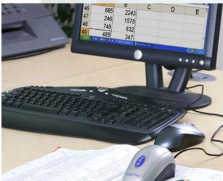
Figure 7b: MonoMouse™ USB works with any desktop or notebook PC. When the software is activated, a pop-up window is launched and the image captured is within that window. The window can be resized with effective change upon the magnification and may be left running alongside other applications. A visually impaired person undertaking office work would find this flexibility useful.
