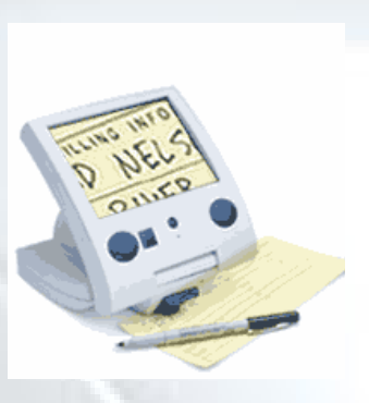
Figure 5a (above): FarView by Optelec: Distance and Near viewing Options. Up to 24x magnification with up to 4 hours continuous use from fully rechargeable battery
