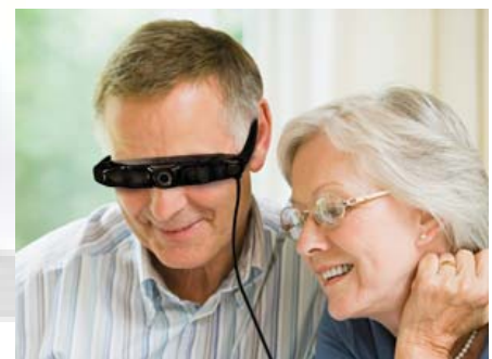
Figure 8 Vuzix SightMate™ is a portable lightweight video magnifier that combines an integrated miniaturised camera and high resolution technology to display near or distant images or text. The 2 mega-pixel camera sensor and 3x optical zoom lens projects onto twin high resolution LCD displays. Battery life is approximately four hours.
